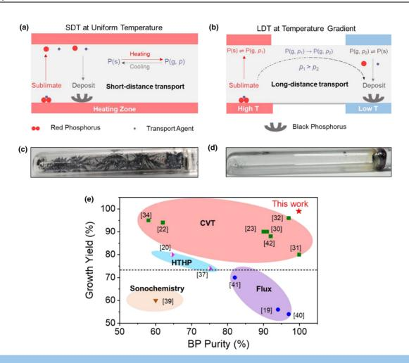
SDT growth of BP under a uniform temperature with the highest growth yield and purity. (a), (b) Schemes of uniform temperature SDT and temperature gradient LDT strategy to grow BP. (c) and (d) Photographs of the as-grown products in the SDT and LDT growth methods. (e) A summary of literature reports on the growth yield and purity of BP grown by various methods.
