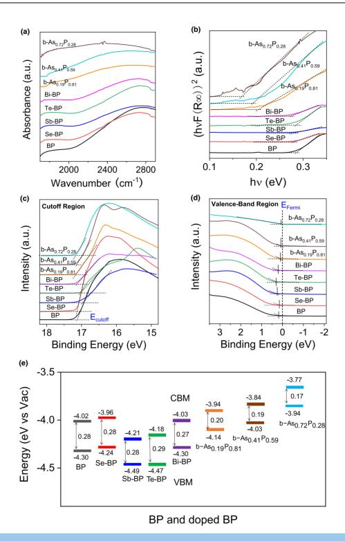
Tuning of electronic properties of BP produced by doping. (a) DRIFT absorbance spectroscopy, (b)  $hv - (hv * F(R_{\infty}))^2$  curves; (c) cutoff region of UPS spectra, (d) Valence-band region of UPS spectra. An offset has been added to the curves for better clarification for (a–d). (e) Energy band alignment of pristine and doped BP materials.
